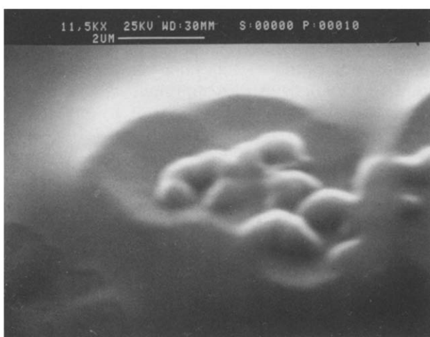
Figure 7 Enamel-like morphology of PPA-C showing evidence of the 'unwinding' of the microspheres
