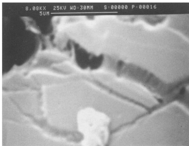
Figure 6 Enamel-like morphology of PPA-A after annealing for 20 h at 393 K
